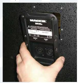
2 Once loosened, the input assembly may be easily removed from the cabinet. Do not completely take the input assembly off yet, as two cables need to be removed first.
